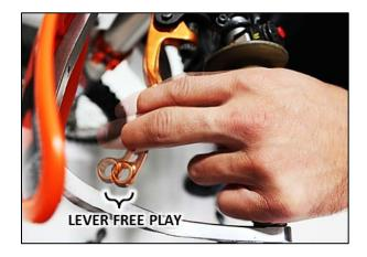
"Free Play Gain" is the increase of lever free play as the auto-clutch engages. This happens when the RPM increase from idle through around 5000 RPM. Free Play Gain is caused by the expansion of
