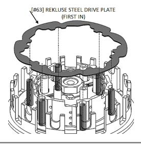
**NOTE:** Proper orientation of the drive plates is *critical* for optimal clutch performance. If you install them backwards, the clutch will still function but will lack proper modulation performance.
