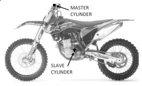
**16.** Starting at the slave cylinder, remove the OEM parts named in the following diagram beginning with the bleeder bolt.
