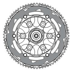
**9.** Install the rest of the clutch pack, noting the number and order of plates shown.
