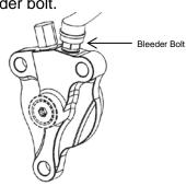
Use a socket and torque the separate bleed screw to 180 in-lbs. (20 N-m) to seat and seal the bleed screw once bleeding is complete.
