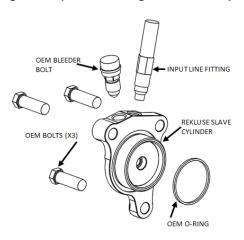
**NOTE:** Some models have a paper gasket and/or O-ring seal. Reuse them if OEM equipped.
