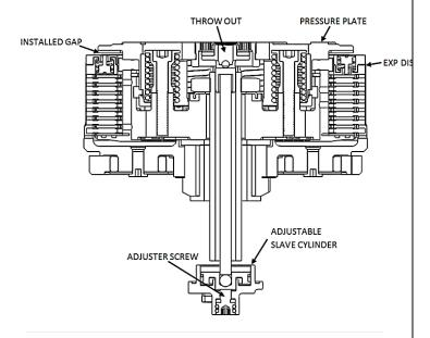
27. Using the long end of a 4mm Allen key, turn the adjuster screw clockwise until it stops under moderate pressure. You are trying to feel for the point at which the throwout will start to lift the pressure plate. This is the "starting point".
