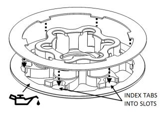
**12.** Install this pressure plate subassembly.
