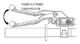
**23.** Using an 8mm wrench, open the bleeder bolt. Air and fluid should come out of the bleed tube. Tighten the bleeder bolt.
