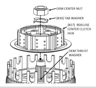
Torque the nut to 50 ft-lb (68 N-m), then bend up both tabs of the tab washer using channellock pliers.
