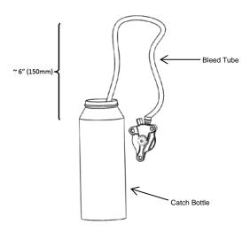
**22.** Pump the clutch lever 3-5 times then hold it against the bar/grip.
